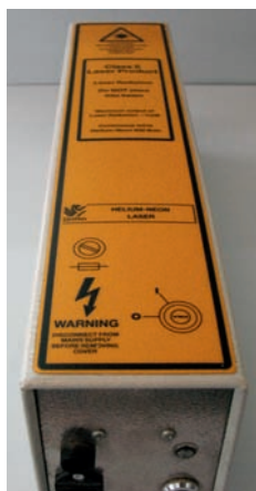
■ Figure 2.28 A helium-neon laser (632.8 nm wavelength)
