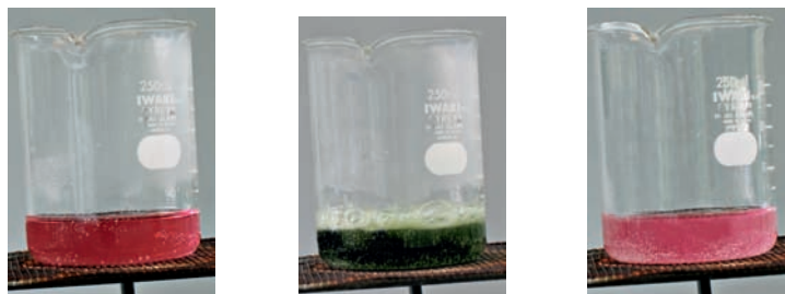
■ Figure 6.15 The reaction between tartrate ions and hydrogen peroxide in the presence of cobalt(II) ions, acting as a catalyst. The pink solution on the left contains cobalt(II) ions, the green solution in the middle contains a temporary green intermediate containing cobalt(III) ions, and the pink solution on the right contains regenerated cobalt(II) ions
