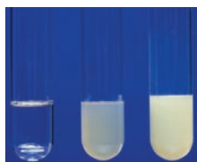
Figure 20.13 Using silver nitrate solution to indicate the release of halide ions during nucleophilic substitution: the white precipitate of silver chloride is yet to appear in the left-hand tube, showing that this substitution is the slowest of the three
