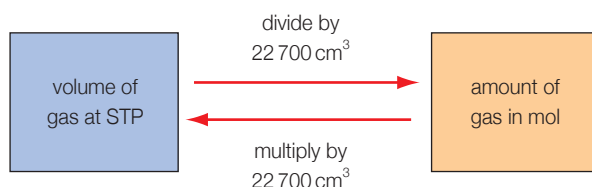
■ Figure 1.47 Summary of interconversions between the amount of gas and volume (at STP)
