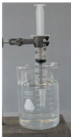
■ Figure 1.51 A sealed syringe of air in a beaker of hot water
