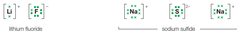
■ Figure 4.28 Lewis structures (electron dot diagrams) for lithium fluoride, LiF , and sodium sulfide, Na_2S
