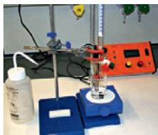
■ Figure 18.15 Apparatus to record titration curves: the reaction mixture is stirred magnetically and the change in the pH recorded on the meter
