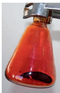
■ Figure 7.4 A sealed flask containing bromine demonstrates a physical equilibrium between the liquid and its vapour
