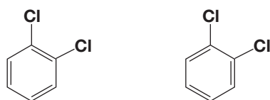
■ Figure 10.49 The hypothetical (Kekulé) isomers of 1,2-dichlorobenzene – in fact the compound has a single, unique structure
