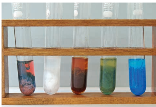
■ Figure 13.69 Precipitates of hydrated transition metal hydroxides. From left to right: cobalt(II), zinc, iron(III), iron(II) and copper(II)
