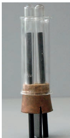
■ Figure 19.14 Electrolytic cell with graphite electrodes and ignition tubes in which any gases released at the electrodes are collected
