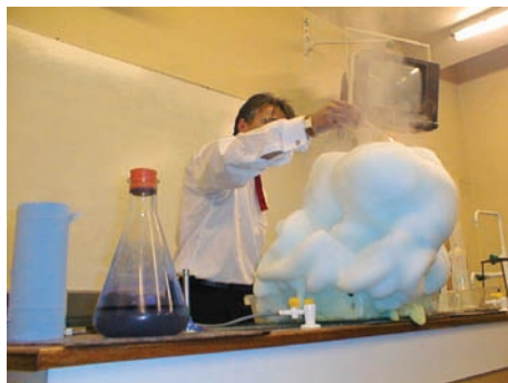
■ Figure 6.14 The production of an oxygen-filled foam from the manganese(IV) oxide catalysed decomposition of hydrogen peroxide (note that the demonstrator should be wearing a lab coat)
