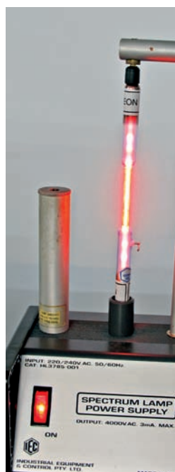
■ Figure 2.42 A high voltage discharge tube containing neon gas at low pressure
