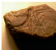
■ Figure 4.12 An impure sample of corundum: a very hard, crystalline form of the ionic compound aluminium oxide
