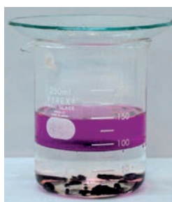
■ Figure 17.4 Iodine dissolved in a mixture of hexane (upper layer) and water (lower layer)
