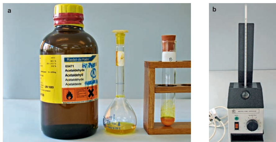
■ Figure 10.79 a The 2,4-dinitrophenylhydrazine test for aldehydes and ketones. An orange precipitate is formed in either case. b A commercial melting-point apparatus
