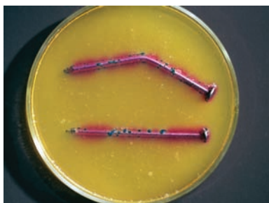
■ Figure 9.32 A rusting nail in the presence of ferroxy indicator (an aqueous mixture of potassium hexacyanoferrate(III) and phenolphthalein)
