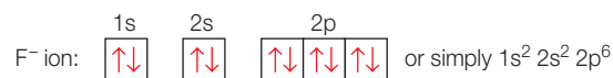
■ Figure 2.64 Orbital notation and detailed electron configuration for a fluoride ion, F^-
