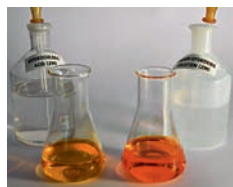
■ Figure 7.13 The equilibrium between chromate(vi) and dichromate(vi) ions in solution can be manipulated by the addition of acid or alkali
