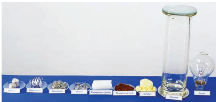
■ Figure 3.2 Samples of the period 3 elements: sodium, magnesium, aluminium, silicon, phosphorus, sulfur, chlorine and argon
