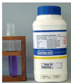
■ Figure 18.11 Universal indicator solution added to a concentrated solution of sodium carbonate: the colour shows that it is alkaline
