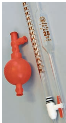
■ Figure 1.63 A selection of apparatus used in a titration: pipette filler, burette and pipette
